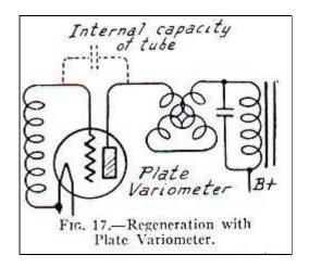
As the variometer's inductance is increased, the feedback through the tube capacity increases so that additional energy is sent back into the grid circuit. Reducing the variometer's inductance reduces the regeneration.
