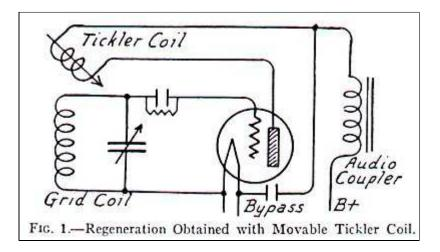
*Tickler Coil Control.*- Fig. 1 shows regeneration obtained by a tickler coil connected in the plate circuit and coupled to the tuned coil of the grid circuit. The construction of the tickler coil unit is shown in Fig. 2. The tuned winding, which is the secondary of a radio frequency transformer, and the primary winding of this transformer are wound on a stationary form in the usual way. The tickler coil is wound on a form which rotates within the stationary form.
