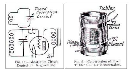
As the regeneration control condenser is tuned more and more closely to the frequency being received, the power absorbed from the grid circuit will increase and regeneration will be reduced.
