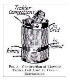
As the tickler is turned to increase its coupling to the stationary coil the effective inductance of the tuned stationary coil is increased. Therefore, the tuning point at which the circuit becomes resonant to a certain frequency will change with changes of tickler adjustment. This is a rather serious disadvantage of this method for obtaining regeneration since a receiver cannot be logged unless a note is made of the tickler coil setting.
