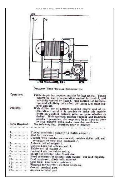
**COIL, TICKLER.**-A tickler coil is a coil electrically connected in one circuit and coupled to another circuit so that energy from the circuit in which the coil is connected may be introduced into the circuit to which the coil is coupled. A tickler coil is used as shown in Fig. 1 to secure a feedback of energy from the plate circuit of a tube to its grid circuit for the purpose of causing regeneration. The tickler coil is connected in the plate circuit and coupled to the grid coil of the tube.
