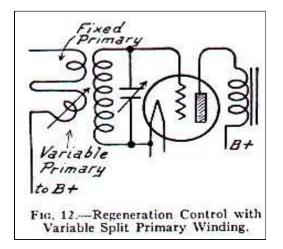
The split primary winding of Fig. 12 has been used for automatic control of regeneration by attaching the movable part of the winding to the shaft of the tuning condenser. More regeneration is always required for low frequencies than for high frequencies, consequently the connection is made so that the two parts of the primary act together for maximum regeneration at low frequencies or high wavelengths.
