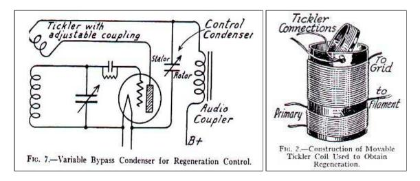
The connections are made exactly as shown in <u>Fig.7</u>. The plate of the tube is connected to the tickler and the other side of the tickler is connected to the stator plates of the control condenser and to the primary of the audio transformer. The rotor of the condenser is connected to either filament terminal of the tube.
